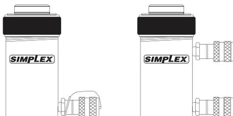
Make hydraulic connections. Use a pump with a release valve or a 3-way valve and one hose for single-acting cylinders. Use a pump with a 4-way valve and two hoses for double-acting cylinders.
