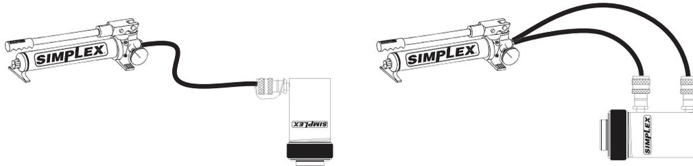
Single-acting cylinders: Position the cylinder so that the plunger is pointed down and the cylinder is lower than the pump. Fully extend and retract the cylinder 2 or 3 times.
